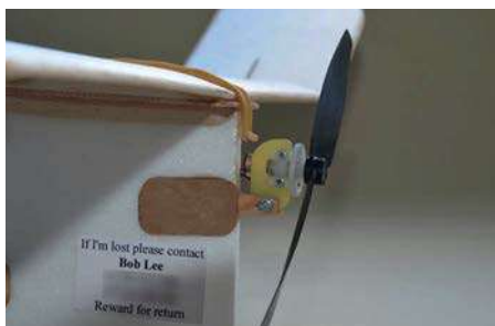
Close up of motor mounting, LH side
